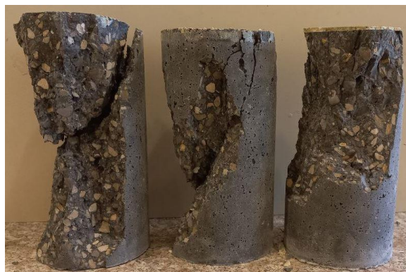
Figure 11. Failure pattern of SCC mixture made with 2% of ONS particles at 28 days.
